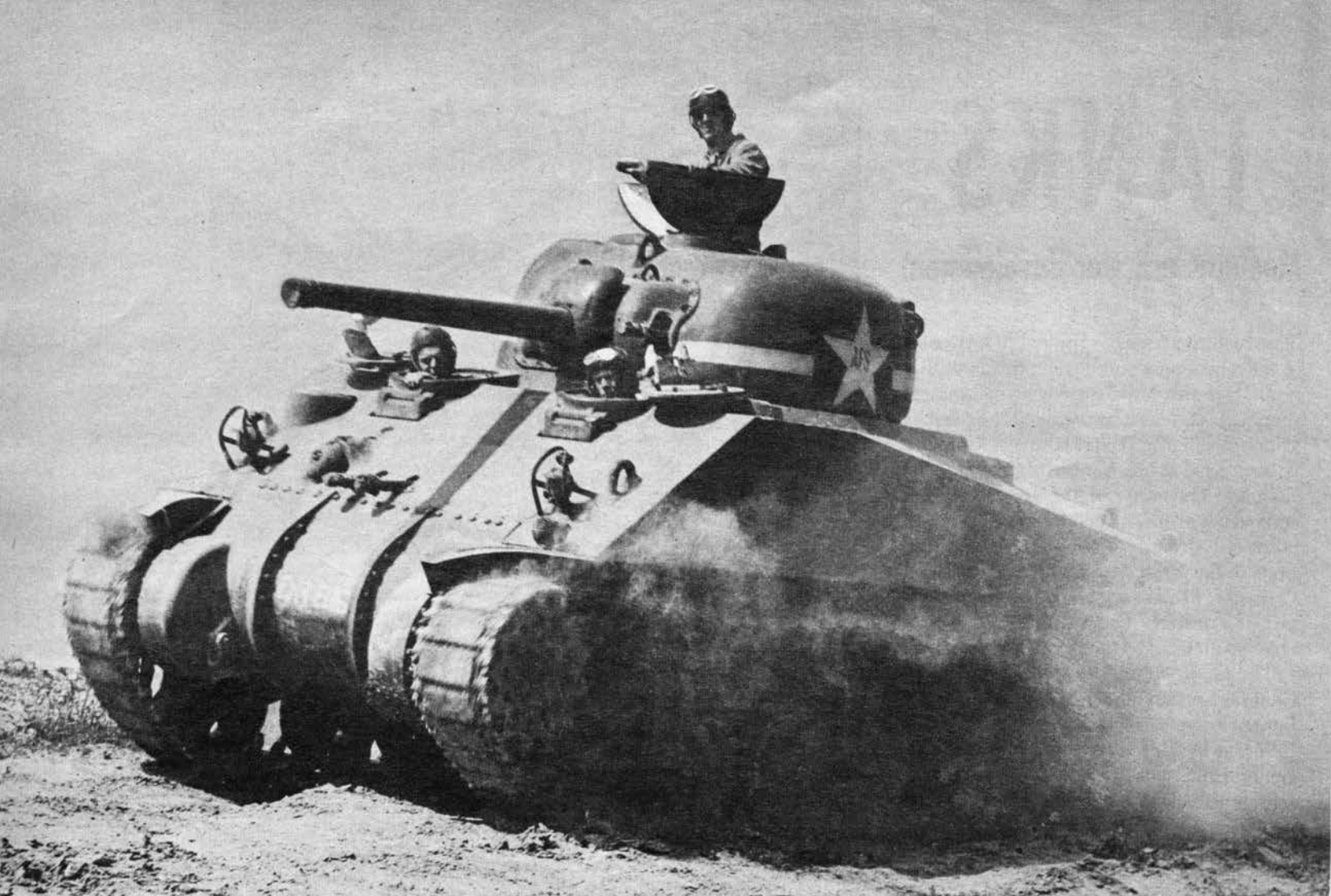
GENERAL SHERMAN M-4 WITH 75-MM. ARMAMENT IS THE STANDARD AMERICAN MEDIUM TANK. ITS TURRET IS LARGE AND ROUNDED; HULL, ANGULAR BUT STREAMLINED
